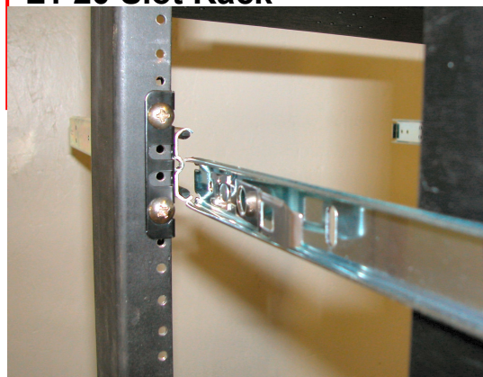
View of chassis being inserted into the side rails.
