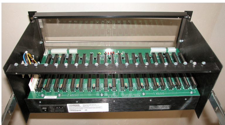
Chassis view with cover removed to allow cards to be inserted.
