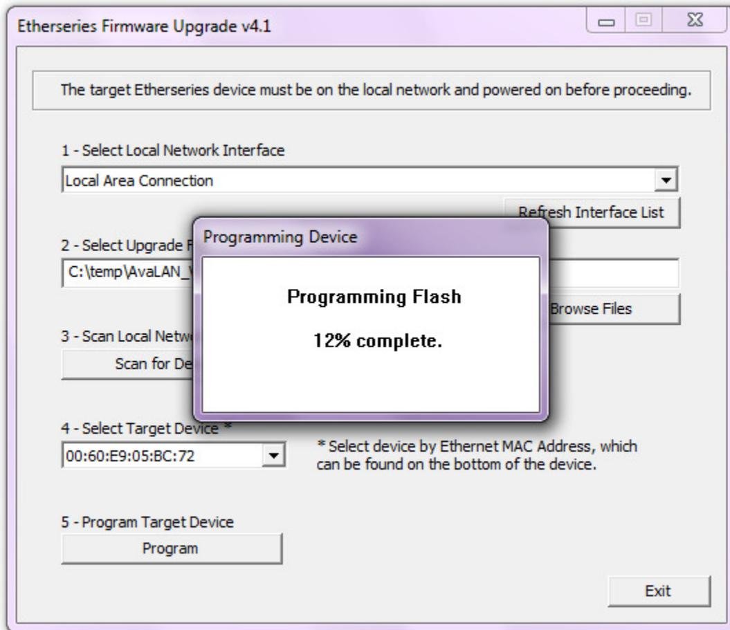
After the AvaLAN flash programming step is finished, the new firmware is verified to confirm that the update was successful.
