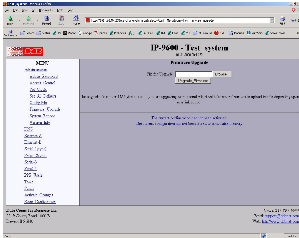
Firmware Upgrade Screen
