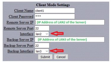
Figure 3 – Client Mode Settings For Path Redundancy
