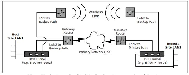
Figure 2 – An Example of Path Redundancy Between Tunnel Devices
