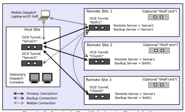
Figure 1 – Configuration for Tunnel Redundancy in a Dispatch Application
