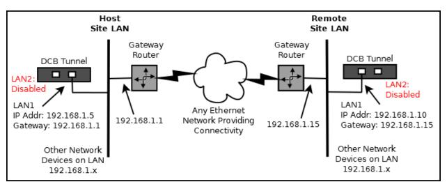
The tunnel devices at either the remote, host, or both may be used in this manner. Figure 1 below diagrams such an arrangement, with sample LAN addresses shown.
